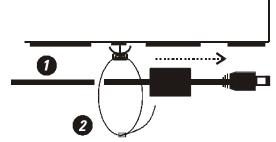
2 Tighten the cable tie until the cord is secure. Do not over tighten.
